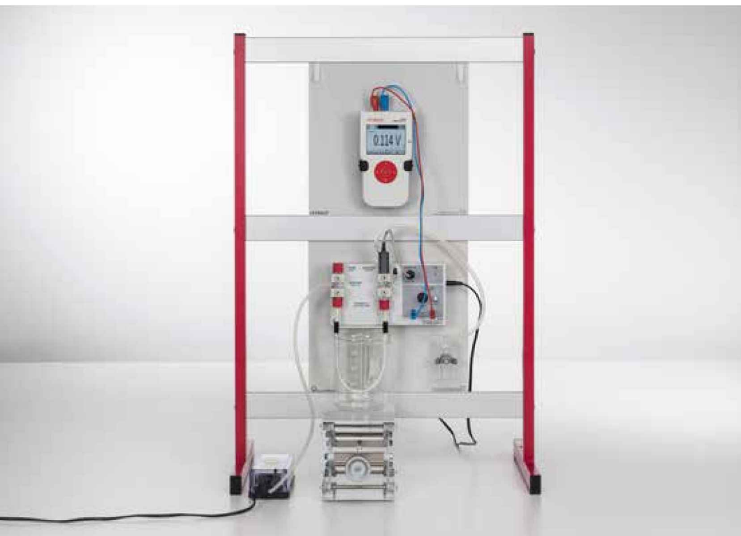
Gas chromatographical separation of alcohols - effect of temperature (C3.2.1.2_p)
